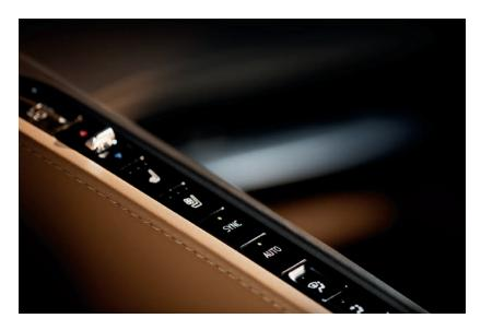
CLIMATE AND SEAT CONTROLS ATOP COCKPIT BUTTRESS
