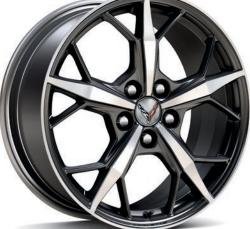
19" X 8.5" FRONT AND 20" X 11" REAR 5-TRIDENT-SPOKE MACHINED-FACE SPECTRA GRAY-PAINTED ALUMINUM WHEELS
