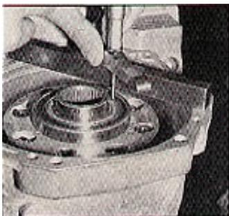
18. To measure the correct end play, place the straightedge tool J-34673 across the face of the overdrive unit and use the depth micrometer J-34672 and
