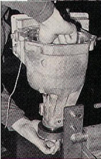
9. (right) Lower the output assembly into the case lining up the oil pump ports and bolt holes. Start all four pump attaching bolts, but don't tighten them yet. First install the driveshaft yoke into the rear of the O/D unit and then tighten the bolts. This will properly line up the pump and shaft in the case.
