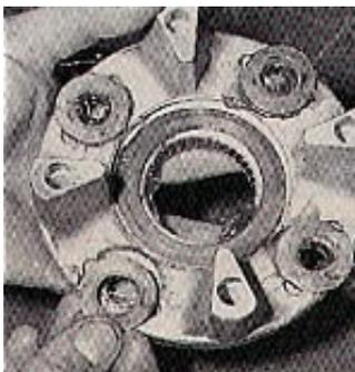
16. Take the annular bearing assembly, turn it over and install the pinion thrust washer and sun thrust washer.
