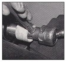
Remove the old rubber mount and install the new polyurethane mount in its place. Install a new clamp on boot and reinstall the tie rod. Stake the inner tie rod end so it won't loosen up.
