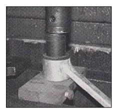
The next step is to remove the shaft from the arm. Then press out the other bushing.
