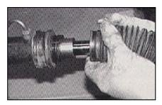
With the rack secured, cut the boot clamp and pull the boot up on the tie rod to expose the inner tie rod end.
