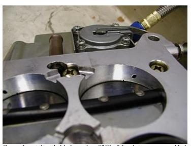
Correctly set throttle blade angle. .020" of the slots are exposed below the blades. Both primary and secondary throttles should be set exactly like this (except Holley – see the BG Setup Paper and Holley Paper for correct Holley secondary idle setting)
