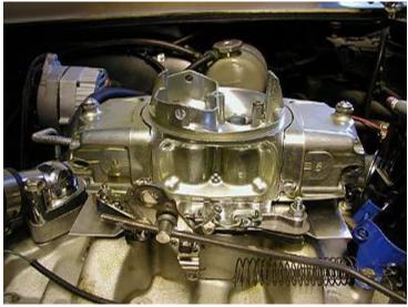
Left side view of completed installation showing dual throttle return springs and shield tucked under carb.
