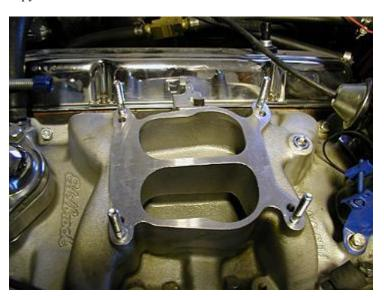
Using the ½" thick insulating gasket under the heat shield requires use of long mounting studs. Note also that the vacuum fitting in the manifold to the rear of the carb has been removed and a flush allen-head pipe plug has been installed to clear the BG rear float bowl and allow installation of the jogged shield.
