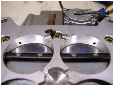
"Out-of-the-box" setting of the throttle blades shows secondary throttle closed completely – there is no exposure of the transition slot on the secondary side. Primary side had massive slot exposure to compensate for lack of adjustment on secondary side.
