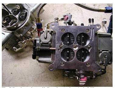
The BG carbs, and most Holleys, have only a single 3/8" vacuum port for connection of the PCV. If you're running power brakes, you can install a "T" system like this to run PCV and brakes. I have made the "T" section short enough that it is hidden under the secondary bowl. This makes a very clean installation. Note twin vacuum nipples coming out of the side of the throttle plate: The forward nipple (right) is ported
