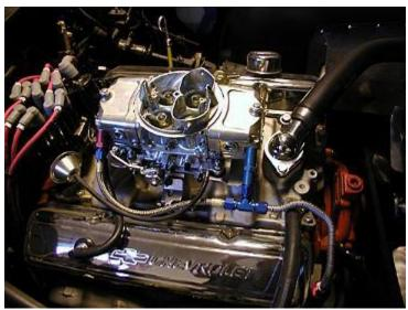
Complete setup bolted up and ready for test run. Note how heat shield clears all components and is nearly invisible. Steel fuel line keeps things safe and clean looking.
