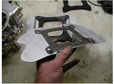
Shields can be made in many ways. Shown her is the custom shield that I use on my own car. It's fabricated from a piece of aluminum sheet stock. Note forward and rear edges bent down to clear accel pump levers.
