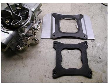
In order for the "jogged" shield to clear the base gasket, the gasket "ears" must be trimmed. Shown here is a trimmed base gasket that will allow the bent shield to fit properly.
