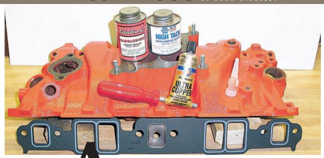
n intake manifold swap is a popular way to improve performance, especially if you stick with GM parts to avoid carburetor-to-air cleaner fit problems (different air horn diameters, choke housing interferences, etc.) and air cleaner-to-hood clearance issues.
