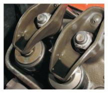
The rocker arm, pushrod socket and valve head are all lubricated with oil during operation. This is extremely beneficial, until you try to adjust the valvetrain during operation. The hot oil splashes out and can make a mess of your engine bay. By adjusting your valvetrain cold, you eliminate the mess and eliminate your chance of getting burned.
