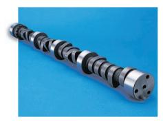
Camshaft operation is more than an open-and-close case. The lifter, and subsequently the pushrod, rocker arm and valve, accelerate at different speeds throughout their operation. Properly adjusting the valvetrain ensures that they are timed appropriately for each event and helps prolong valvetrain life by utilizing the camshaft's ramps to open and close the valve without slamming the valve shut or hammering the valve head when opening.
