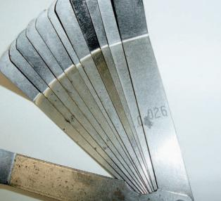
Clearances should be checked with a feeler gauge between the head of the valve and the rocker arm. Depending on the engine displacement and camshaft used, one of the techniques listed will bring your solid-lifter camshaft into proper adjustment for peak performance.
