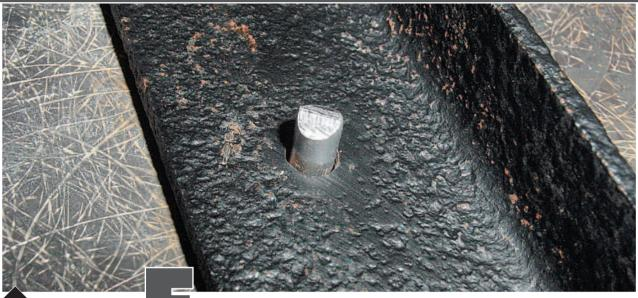
Here's a rivet in place, ready to be set. It has been trimmed so about 3/8" of the shank remains above the steel part.
