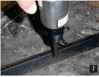
**6** Everything you need to set body rivets — air hammer, rivet-setting shank, and pressure regulator. Just use something solid to back up the flat head end of the
