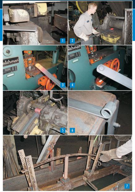
For C1s, steelmakers no longer produce the grooved raw material originally used, so C1 owners should focus on having their original springs re-arched. For C2/C3s, the SAE 5160 alloy steel (premium leaf spring steel used by Eaton for ALL of their springs) is no longer produced in the original .214" and .194" thicknesses, so the next-closest thicknesses are used, with the spring camber adjusted to maintain original ride height.
