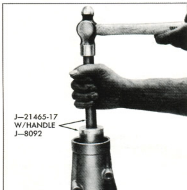
Fig. 11—Removing and Installing Rear Extension Bushing
