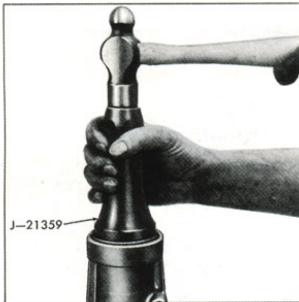
Fig. 12—Installing Rear Extension Seal
