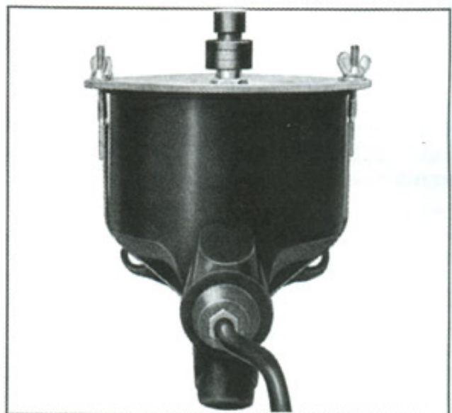
Fig. 30—J-21994 Pressure Bleeder on Master Cylinder
