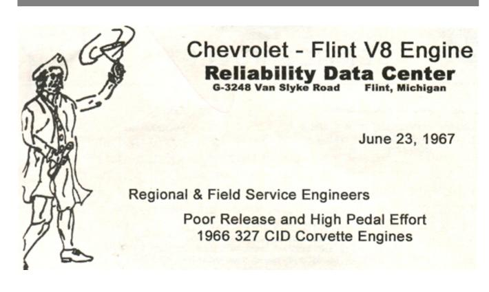
Recent investigation of poor release of clutch, high pedal effort and disc wear has isolated the condition to the clutch fork retainer tangs interfering with the clutch housing boss provided for the ball stud which causes a reduction in fork travel.
