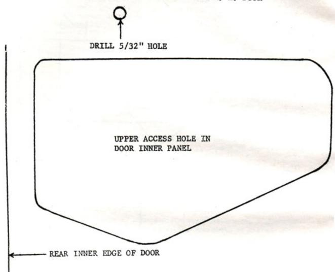
ALIGN TEMPLATE TO REAR INNER EDGE OF DOOR AND ACCESS HOLE EDGES TO LOCATE WATER SHED HOLE LOCATION
