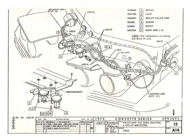
The schematic below shows the position of the headlight vacuum hose along the driver's side inner fender well:
