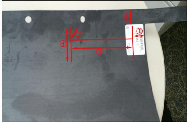
Place the new front compartment air deflector on a surface that can be used to cut on. Mark the dimensions of 25.4 mm (1 in) (1), 19.05 mm (.75 in) (2), 152.4 mm (6 in) (3), 50.8 mm (2 in) (4) as shown in the illustration above and cut using a box cutter.
