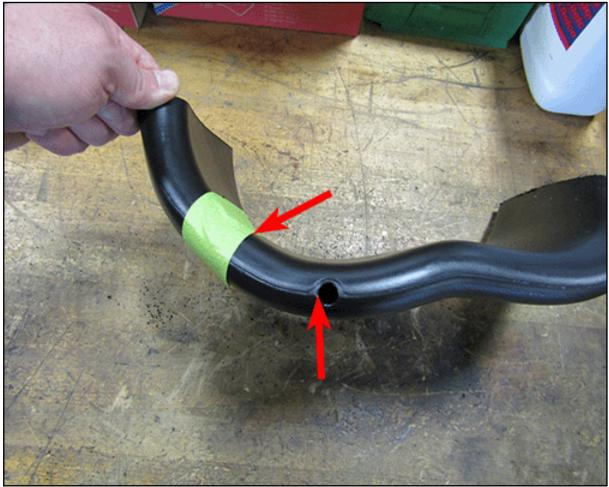
1. Measure 50.8 mm (2 in) up from the top of the hole. Mark and cut using a hack saw.
