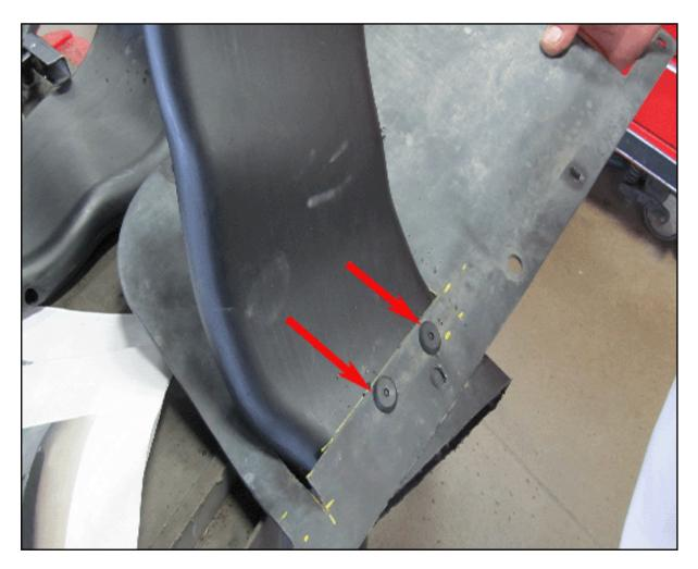
Place the cut duct into the slot. Make sure it comes out of the slot 25.4 mm (1 in). Using a 17/64" drill bit, drill 2 holes through the deflector and duct and rivet together.
