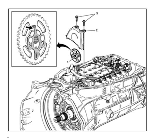
**Note:** Ensure the driven sprocket locking tab is in the unlocked position before installing the sprocket. The driven sprocket locking tab is located on the back of the sprocket and faces the pump.
