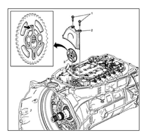
1. Using the DT-48285 Torx Plus socket, remove the two fluid baffle bolts (1) and fluid baffle (2). Discard the bolts.
