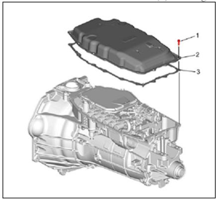
**Note:** The fluid pan gasket is reusable. Inspect the gasket to determine if it may be reused. If the gasket is stuck to the case or pan, it should be replaced.
