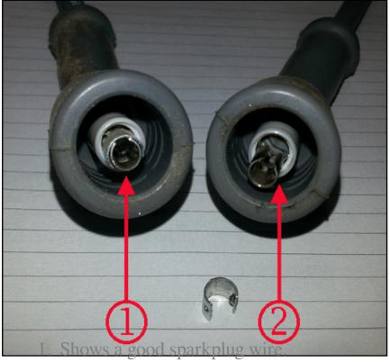
2. Shows the wire with the C clip missing.
