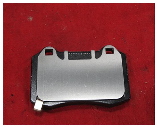
5. (Chevrolet SS Models Only) Apply a rectangular shape of copper paste in the center of the spacer before installing on the back of the pad.
