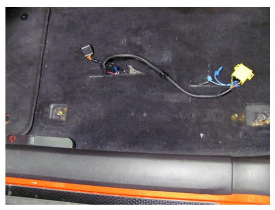
4. On the vehicle harness, pull the harness from under the carpet, to the front location as shown.
