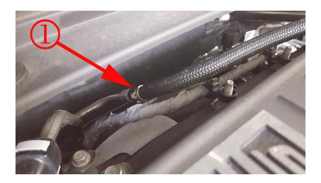
These pictures above shows the chassis fuel feed pipe for the LT4 supercharged ZL1 Camaro.
