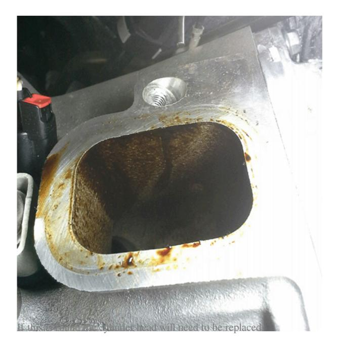
For coolant entry at the liner to deck face casting of the cylinder bore.
