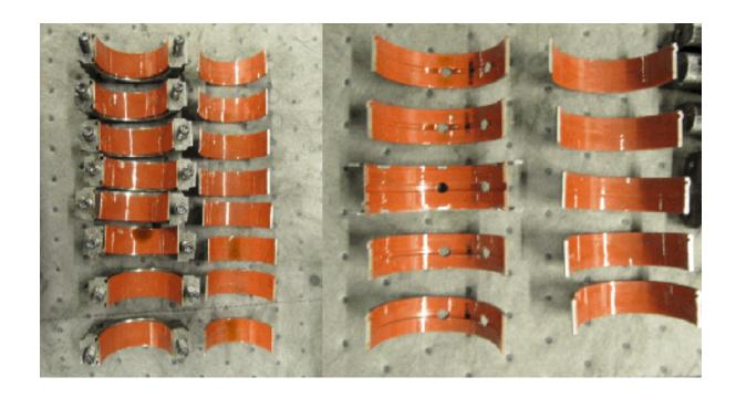
Inspect thrust bearing for wear on one side and crankshaft on that "mating" surface.
