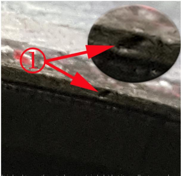
It is hard to see the actual source (pin hole) but it usually streams down the liner so that you can see it with a borescope.(Sometimes) The top of the piston will be steam cleaned.
