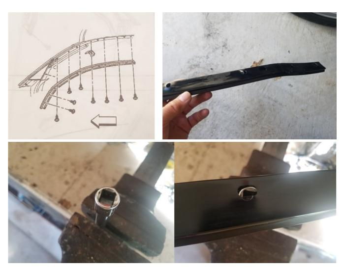
**4.** Carefully clean with 3M adhesive remover 08984 and remove dimples from metal retainer. Use a 3/8 drive extension mounted in a vise to set part on. Then carefully hammer to flatten part.
