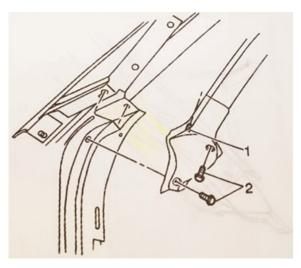
**32.** Close the door with the window up to hold the weatherstrip in place while adhesive cures.
