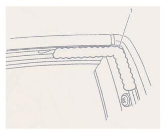
**27.** Apply three parallel 2 inch long beads of sealant (1) to the forward end of the door opening weather strip retainer and to the rear edge of the reveal molding.
