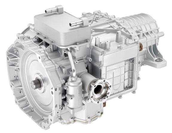
**TIP:** The DCT requires a special transmission fluid to maintain performance and durability standards. ACDelco DCT FFL-4 automatic transmission fluid is recommended. Do not use any other type of fluid. Total capacity is 11.62 quarts.
