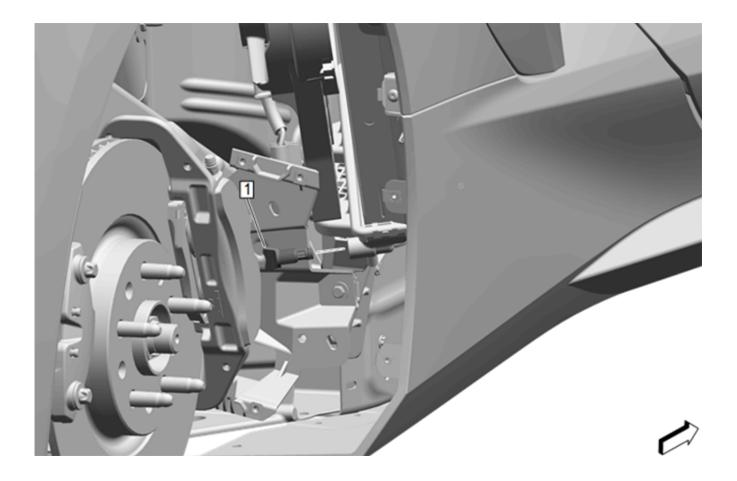
The auxiliary radiator inlet hose connectors and hose caps for each auxiliary radiator are located at the front of the vehicle on each side of the front compartment. (Fig. 4) The front compartment rear access cover and front sight shield must be removed.
