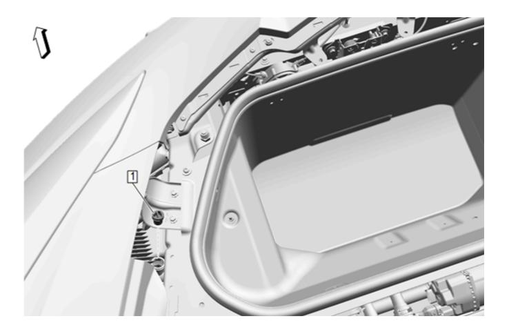
The radiator inlet hose connector cover, located at the rear of the vehicle, uses a hose retainer. (Fig. 5) Disengage the hose retainer to remove the connector cover.
