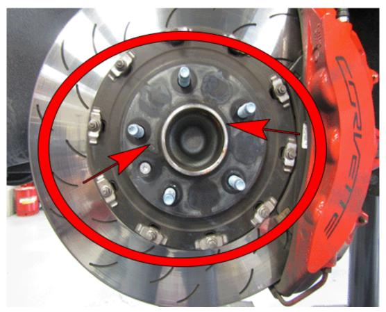
• Using 3M red Scotch-Brite 7447 pad or equivalent with approved brake cleaner (ex. Part number 19370705 (U.S.), 88901247 (Canada)), wipe the wheel mounting surface of the rotor (brake rotor top hat) and the wheel pilot at the center of the
