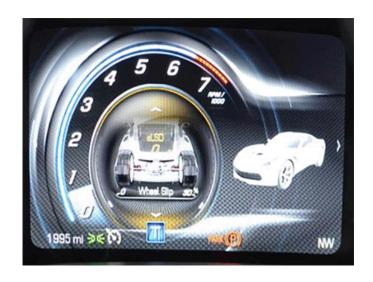
Photos of the Camaro and Corvette DIC screens are shown in the graphics above. This bulletin will provide a general overview of the functions and operation of the eLSD system in these vehicles.
