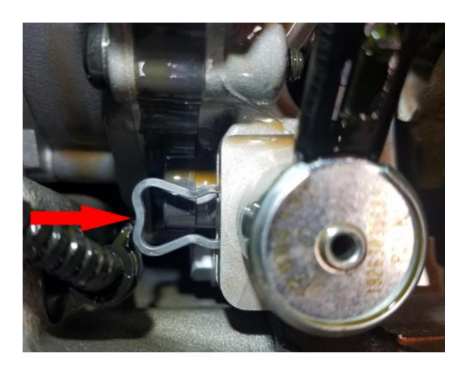
**Important:** Do not use any tools to tap the pressure control valve into place. Only install the pressure control valve by pushing on the body of the valve by hand.
