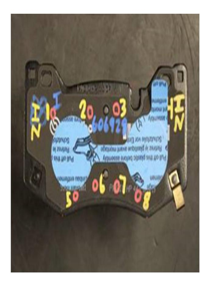
To apply the paste correctly, the pads must be removed from the calipers. See the photo below for an example of what the front brake pads look like once they have been separated from the caliper pistons.
