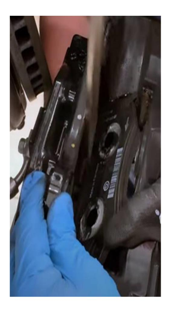
This is normal when the front pads have been removed. When this has been done, remove as much of the remaining tape residue as possible. Then, apply the copper paste as directed in the bulletin. Once the copper paste has been applied correctly to the front brake pads, simply reinstall them into the calipers. There is no need to replace the front brake pads during this service because of the double-sided tape.
