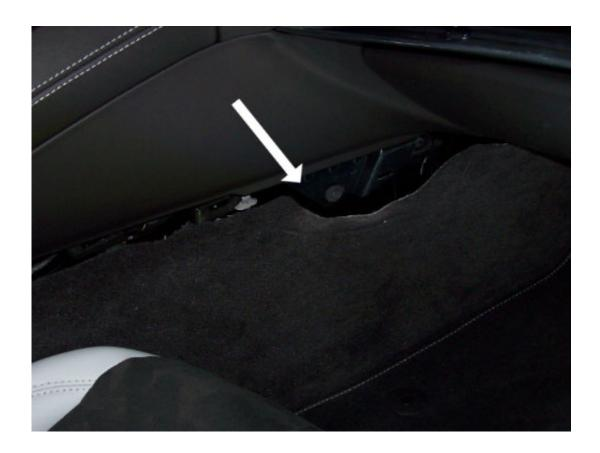
2. Pull back the carpet in the location shown to gain access to the A/C Evaporator Drain Tube.
