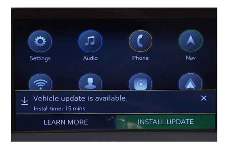
The new Vehicle Intelligence Platform (VIP) electrical architecture, introduced on some 2020 and 2021 model year vehicles, powers a new electronic system that is capable of managing up to 4.5 terabytes of data processing power per hour, which is a fivefold increase in capability over the previous Global A electrical architecture. On vehicles using the VIP architecture, virtually all modules can support OTA updates, which means that the OTA software is not only for the infotainment system.
