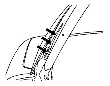
Remove the weatherstrip retainer and the B-pillar exterior molding. Seal the void with GM RTV Silicone Rubber Sealant-Black, P/N 12345739 (in Canada, use P/N 10953541).
