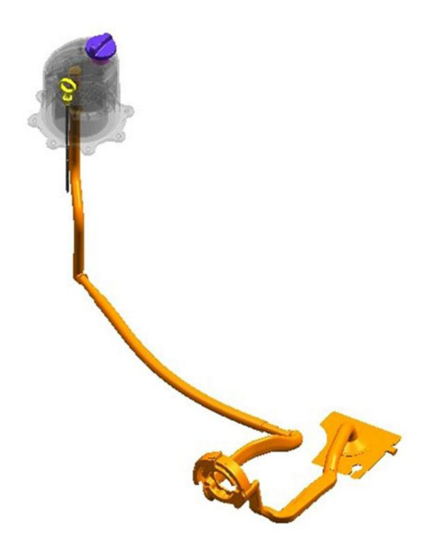
The oil is directed to the top of the reservoir, where it is allowed to spill onto a spiral-shaped baffle. Crankcase gases and air are separated from the oil and are returned by the PCV system to the engine, where they are burned. The deaerated and conditioned oil collects in the bottom of the reservoir, ready for use.
