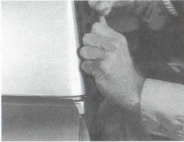
Stretching lower portion of weatherstrip downward
