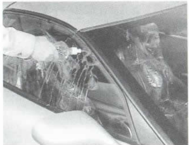
Leaks ahead of the blow-out clip require tip-in adjustment.
