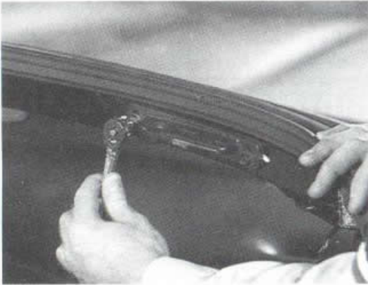
Loosening latch striker bolts
