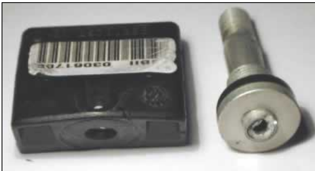
Sensor ruined by tire mounting equipment
