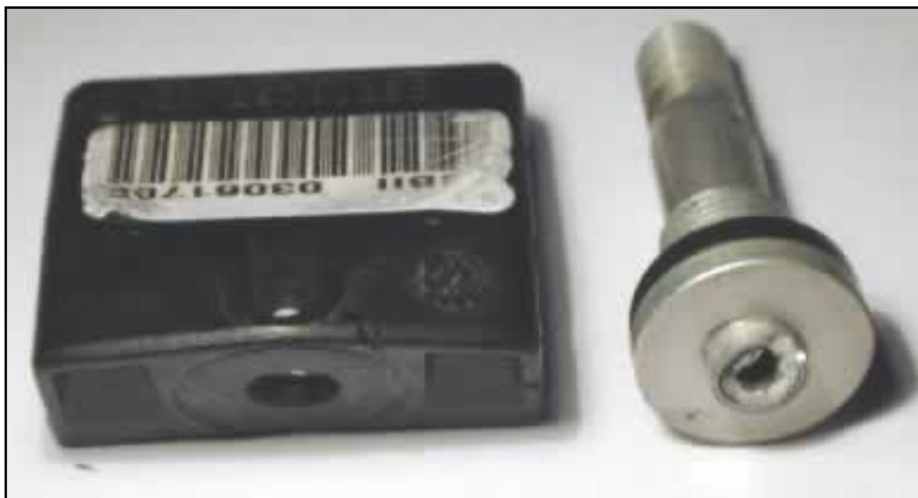
Sensor ruined by tire mounting equipment
