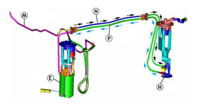
**TIP:** The pressure regulator is in the fuel tank, not on the fuel rail on the engine. This type of fuel system is called returnless, or demand. This means that
