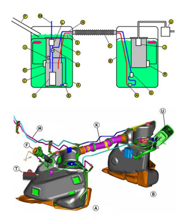
Each tank contains a sensor module, which includes a float and resistor card.
