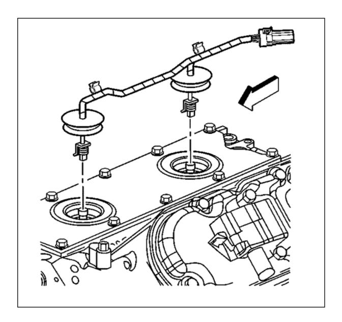
• Remove the wiring harness assembly from the knock sensor.
