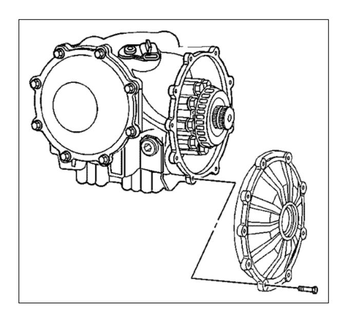
5. Install the differential cover (right) to the differential.
