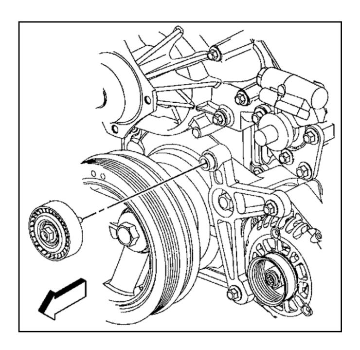
A new idler pulley assembly is available with a thicker dust shield to prevent the distortion of the dust shield. The previous dust shield thickness is 0.61 mm. The new dust shield thickness is 1.37 mm.
