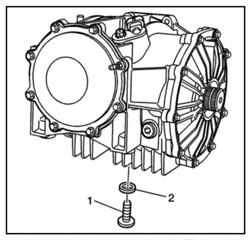
23. Install the drain plug (1) and washer (2). Tighten Tighten the drain plug to 35 N·m (26 lb ft).
