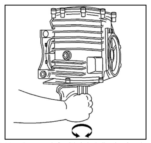
16. Move the output shaft - right in both directions in order to measure the gear backlash. Measure the backlash in two to three locations. Refer to Rear Axle Specifications.
