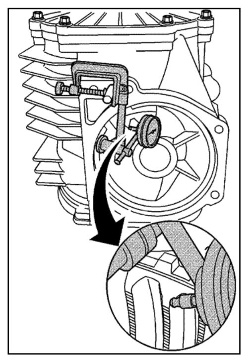
14. Install the J 8001 onto the transmission stud. Position the tip of the dial indicator against the center of the ring gear tooth surface.
