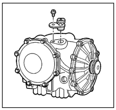
22. Install the vehicle speed sensor and bolt. **Tighten** Tighten the bolt to  $25~{
