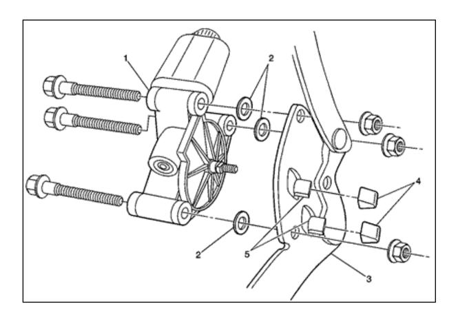
Install one washer (2) between the left headlamp door motor/actuator (1) and the mounting bracket (3) at each of the three attaching bolt locations. Also replace the insulator (4) on each of the two mounting bracket travel stop tabs (5) as shown. For information on headlamp motor/actuator removal, see the Headlamp Motor/Actuator Replacement procedure in the Lighting sub-section of Body & Accessories in the appropriate Service Manual.
