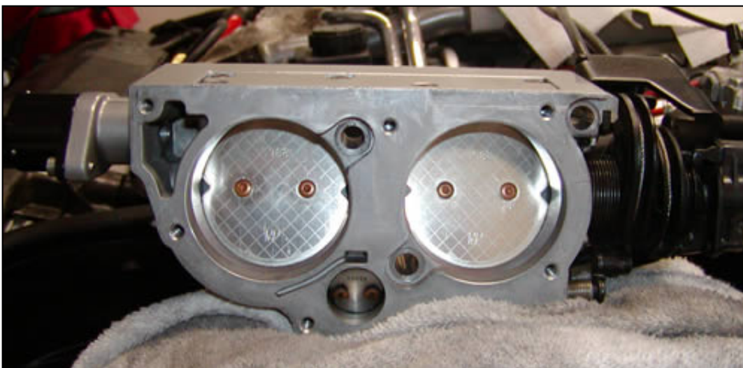
In the center of the throttle body, at the bottom, you see the primary throttle valve which is 22 mm (0.87 in.) in diameter. Above are the two larger secondary valves which are 59 mm (2.32 in.).
