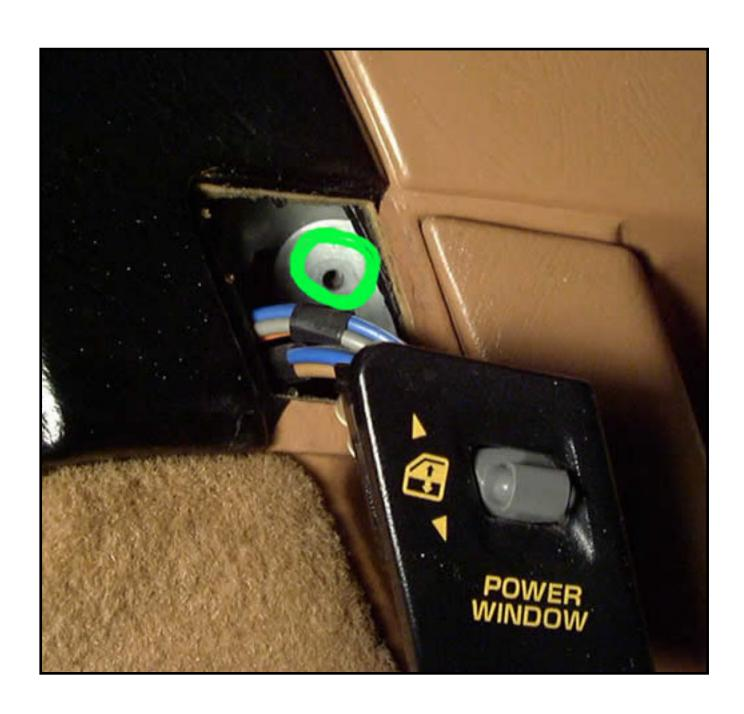
This is a closer shot of the three behind the door handle area. You'll need to pop out the light to get to the top one, and remove the plastic door lock slider piece to get the bottom one:
