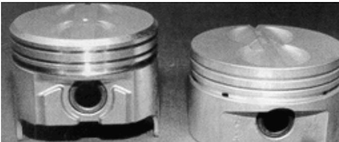
The piston for the 350 LT1 is a special, lightweight flat top with four valve reliefs. The piston for the 265 (left) looks like a smaller version of a 305.
