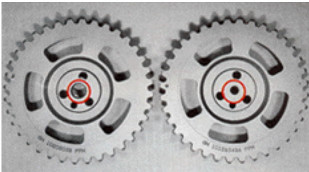
There were two cam gears used on these engines. The early ones (right) had a small hole with 16 splines for the distributor drive shaft while the later ones had a larger, unspined hole.
