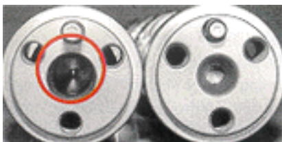
The early cam (1992-'94) had a small, tapered hole and a short dowel pin (right). The later cam (1994-'97) had a deep pilot hole for the distributor shaft in the center and a long dowel pin that was used to drive the distributor.
