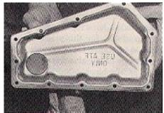
31. Apply a bead of RTV sealant to the oil pan flange and assemble wet. Install pan bolts and torque to specifications.
