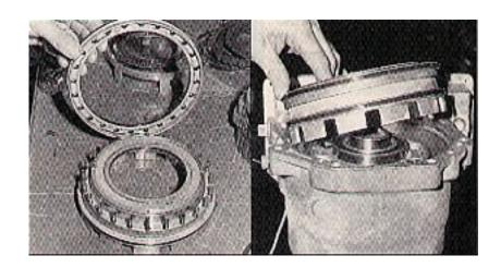
22. Install the accumulator cushion piston onto the accumulator piston and install assembly into case. Reinstall large snap ring in case making sure oil feed hold in lower right side of case is not blocked by the snap ring. Place seal protector J-34621 on input sun gear, install adapter plate sun gear seal with tool J-3423 and adapter plate O-ring, then install the adapter plate. Apply a light coating of RTV sealant on the adapter plate bolts and tighten to specifications.
