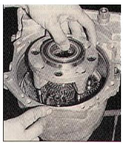
17. Lower the assembly onto the direct drum bolts. The assembly should go on easily if the gears are timed correctly. Install 4 new retaining nuts and torque to specs. Check for lash in all 4 pinion gears, which indicates they are correctly timed.
