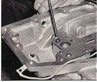
(right) Install second check ball on separator plate.
