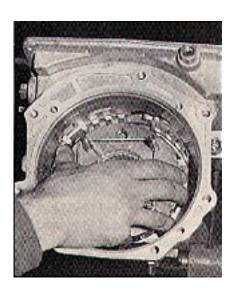
12. Assemble the direct clutch drum, thrust plate and bolts. Once all the bolts are installed all the way, secure them in place with a rubber band and lower the drum onto the direct clutches and plates, rotating it back and forth until it seats home. Remove the rubber band.
