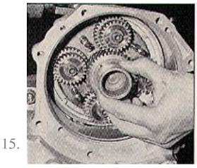
Install the assembly onto the output shaft.
