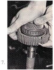
Install the direct clutch hub, then a hub thrust washer, then a hub thrust bearing and another hub thrust washer.
