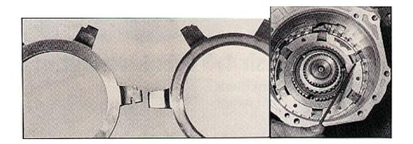
3. The old-style direct thrust washer (above right) was replaced in mid '85-early '86 with the revised washer on the left. Note the special locking tabs on the fingers that keep the washer secured to the direct piston. The problem with the old-style washer was that it would rotate from side to side and notch into the side of the case and prevent the piston from applying or releasing all the way, causing premature overdrive clutch failure.
