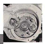
14. Install and time the proof gears opposite each o installed with their many shaft thrust washer or
