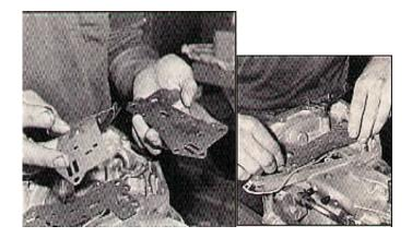
24. <u>Install a new gasket on both sides of the separator plate and position on case.</u>
