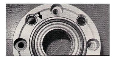
4. The annular bearing was revised in 1986 and was improved to withstand side loading on the bearing. Note the "Thrust Here" (arrow) stamped on the outer race. The early bearing was prone to failure and made a growling noise in direct drive but not overdrive. If your unit has an early direct thrust washer or annular bearing replace them with the newer versions.
