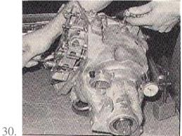
To measure the clutch pack clearance, remove the first 1/8" pipe plug from the left side of the 0/D unit. Install air line fitting J-34742 into pulg
