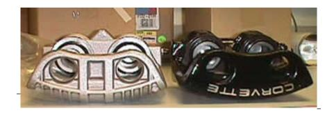
Another view of the top of the calipers showing the difference in ribs.
