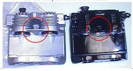
There are a couple of differences noticeable in this pic. First, the ribs on the top of the calipers. The J55 has more ribs but they are thinner than the ribs on the GS. Second, notice that the triangle shaped leg on the J55 caliper is not present on the GS.
