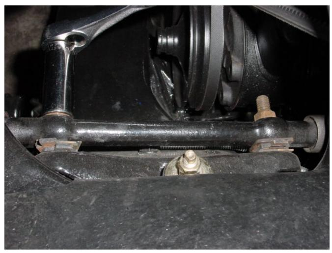
2. Put your floor jack under the frame rail just below the door. Lift the car just enough to take some weight off the front suspension. This will allow you to remove the nuts holding the upper a-arm cross shaft in place.
