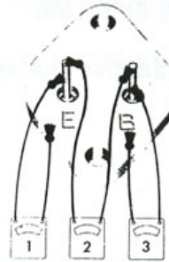
Figure 15—Checking Transistors TR-1 and TR-2.
