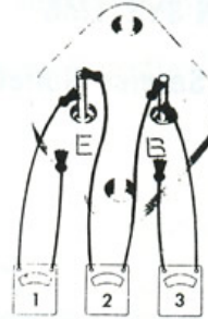
Figure 15—Checking Transistors TR-1 and TR-2.
